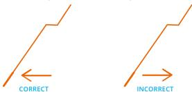
For exposed edges use water and a 50mm brush (or sponge) to clean away all remaining adhesive. Do not leave a groove between the moulding and the wall, as this will show up when painted.
